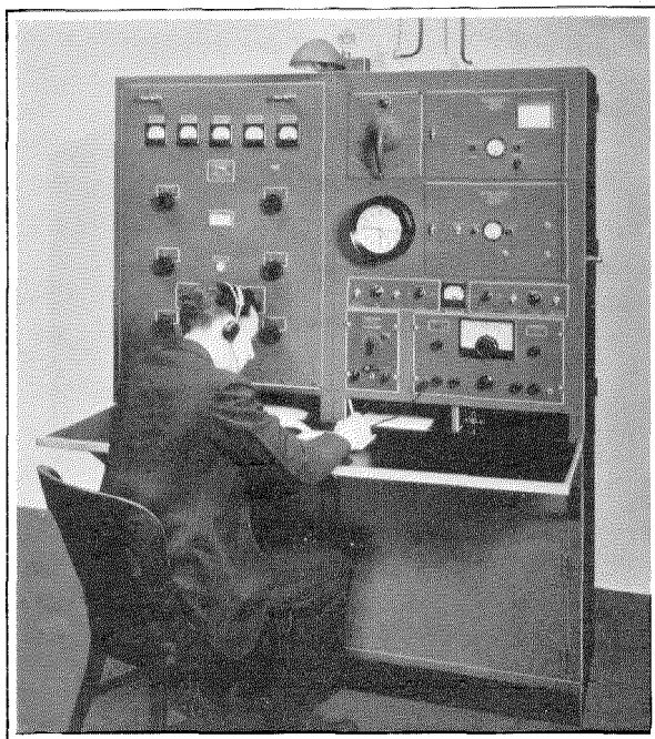
Marine Radio Unit for Cargo Vessels. Developed by the Federal Telegraph Company.
